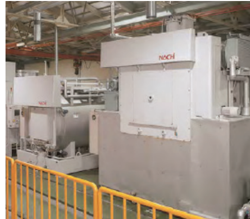
Vacuum carbonizing furnace, vacuum degreasing washer, coating equipment and coating process
