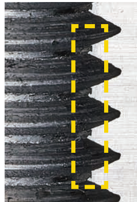
Detailed view with burrs along threads
