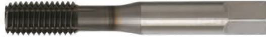
Forming TAP with DLC coating can be used in Aluminum Alloy, Die Cast Aluminum and Copper.
