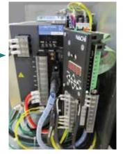
The rotary switch has 1~9 and A~F channels. It is also available to select 16 patterns by setting parameter. (Manual operation mode)
